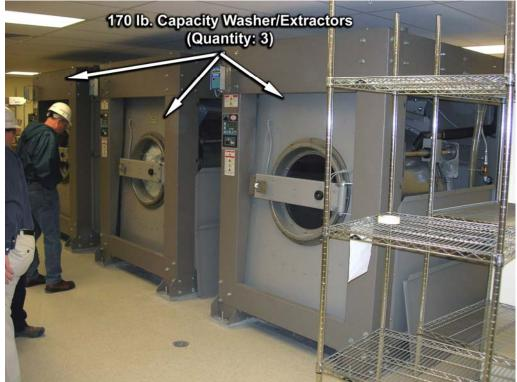
Figure 2: 170 lb. capacity washer/extractors as initially installed.
