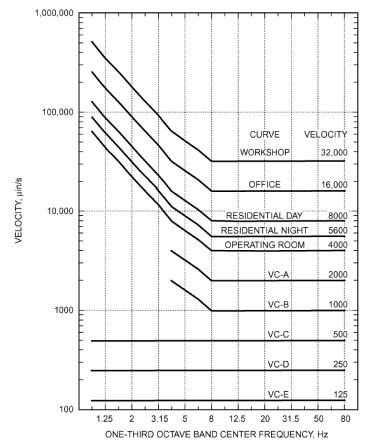
Figure 1: ASHRAE suggested vibration criteria for occupied buildings<sup>2</sup>.
